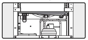
**Step 9.** Lift the unit and place it near the wall opening to route electrical wires through appropriate knock out and drain hose through hole.
