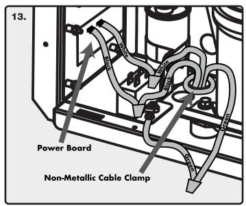
**Step 14.** Tuck the electrical wires in and reinstall electrical cover with its two screws using 1/4" hex nut screwdriver. Be sure none of the electrical wires are pinched.
